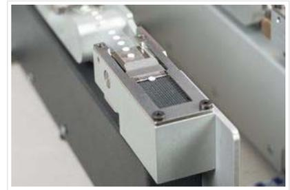
In addition to effective pressure compensation, the mini PCS from Schreiner ProTech delivers reliable protection against intrusion of liquids and dirt for the air conditioning control unit from First Sensor. Mini PCSs are dispensed via the Slimline Label Feeder from pb tec solutions.
